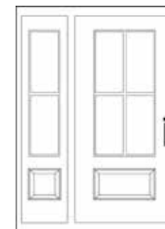
Prehung 4/0 Single with 1 Sidelite (on either side) 51.5" x 82" *
