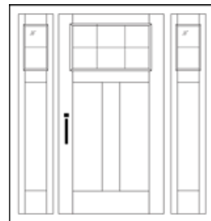
Prehung 5/0 Single with 2 Sidelites 65" x 82" * 5/0 & 6/0 are Prehung on Fusion Frame Composite Jamb
